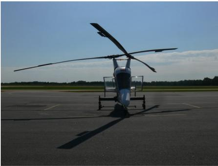
We didn't know whether to greet the visitor or call our pest control guy when the K-MAX 'copter landed at PXE. The aerial truck can lift 6,000 lbs, which is more than the helicopter's own empty weight! Used primarily for logging and firefighting, the K-1200 was enroute to set high-tension electrical towers.
